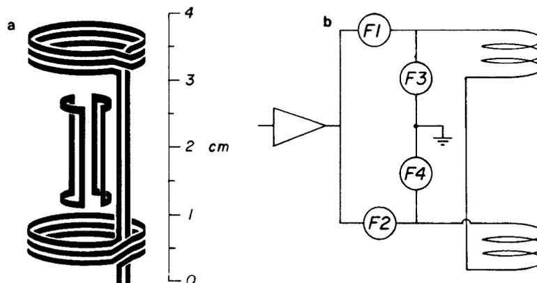
FIG. 1. (a) The geometrical arrangement of the field gradient coils with respect to the radiofrequency NMR coil (shown for simplicity without input leads). (b) Switching circuitry for reversing the polarity of the gradient coils and for damping the ringing after the pulses. During the gradient pulse either the field effect transistors F1 and F4, or F2 and F3, are conducting; after the pulse F3 and F4 are conducting.
