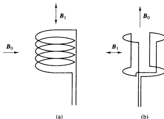
In the figure above (a) corresponds to the solenoidal coil design used in electromagnets and sometimes in solid-state NMR and (b) corresponds to the 'saddle-coil' design commonly used with superconducting magnet systems
