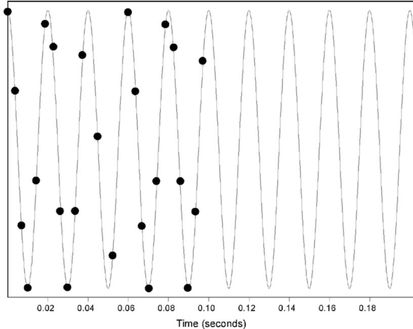
In the ADC, the amplitude of the analog (continuous) signal is sampled at regular intervals.
