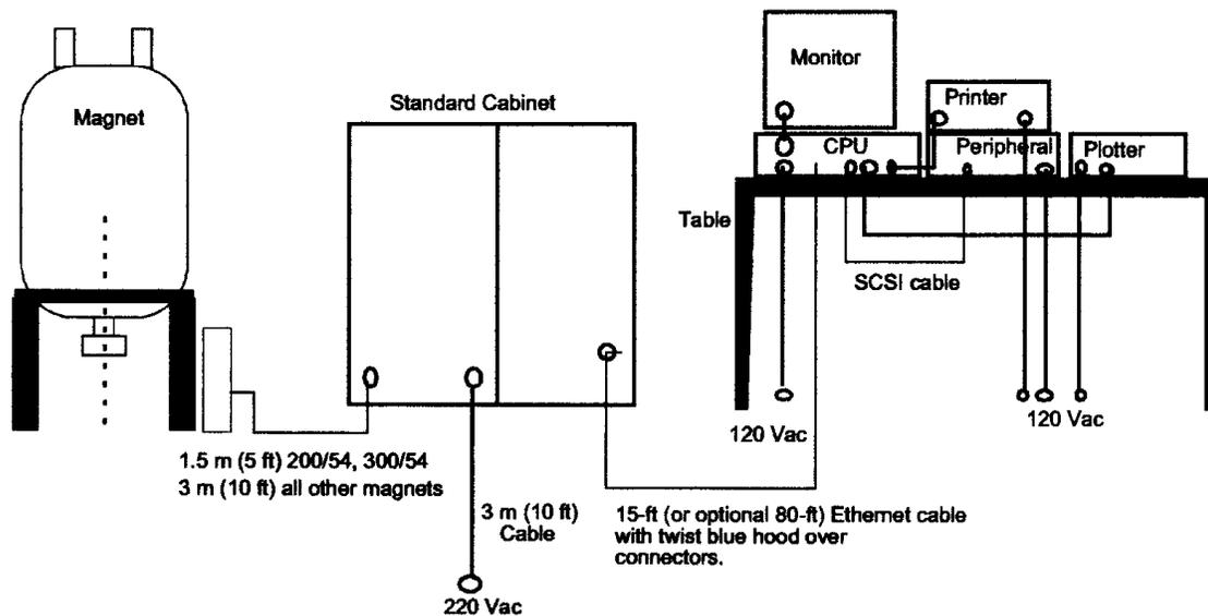
The NMR spectrometer system consists of the following components:
