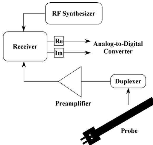
The receiver section provides several levels of amplification including up to 60 dB at the software control level (**gain**).
