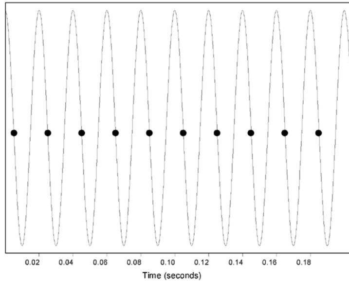
The inverse of the dwell-time is called the sampling bandwidth or the *spectral width*, and its value determines the range of frequencies that may be accurately represented.
